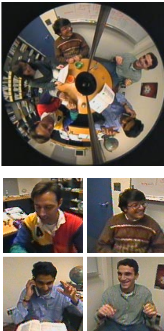
Figure 6: Software generation of perspective images (bottom) from an omnidirectional image (top). Each perspective image is generated using user-selected parameters, including, viewing direction (line of sight from the viewpoint to the center of the desired image), effective focal length (distance of the perspective image plane from the viewpoint of the sensor), and image size (number of desired pixels in each of the two dimensions). It is clear that the computed images are indeed perspective.
