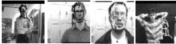
Figure 9: Face finding with learned representations for three scales. The mismatch (right) is caused by the person's unusual arm position.
