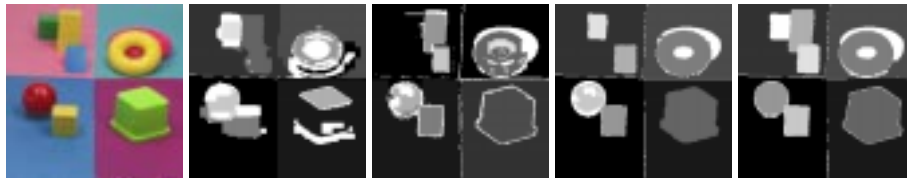
Figure 3: Segmentation results for the split and merge method differentiated for the various color models RGB , S , rgb and l_1l_2l_3 computed from the recorded color image shown in Figure 3.a. a. Color image. b. RGB -segmentation result. c. S -segmentation result. d. rgb -segmentation result. e. l_1l_2l_3 -segmentation result. Note that only l_1l_2l_3 produce region edges corresponding to material transitions.
