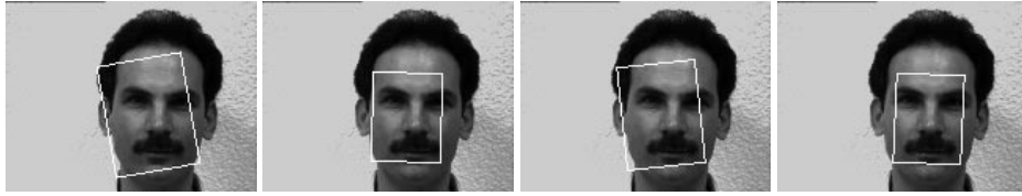
Figure 5: The images show the 1st, the 2th, the 4th and the 8th (final) step of the gradient descent method optimizing the parameters of a superwavelet. The top left image shows the initial values with 10 px. off from the true position, rotated by 10^\circ and scaled by 20%. The bottom right image shows the final result. As superwavelet, the GWN of figure 1 was used.
