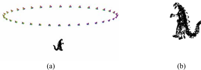
Figure 2: Circular projective reconstruction of the dinosaur sequence. (a) Recovered camera positions and 3D reconstruction of the dinosaur. (b) Another view of the dinosaur 3D reconstruction.
