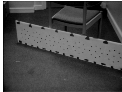
Figure 3: Test group patterns shown at -30 degree trajectory and 30 degree elevation angles, captured using a Hitachi KP-111 surveillance camera placed 6 metres from the target.
